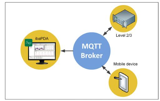
Via the outputs of the MQTT interface, *ibaPDA* can send data to the MQTT broker
