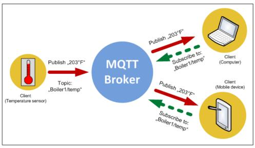
Concerning *ibaPDA*, this means that *ibaPDA* is positioned as an MQTT client that can send data to the MQTT broker and receive data from the MQTT broker.
